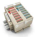
The unique modular concept can be tailored to every type of machine. The potential distribution terminal blocks AAP are successful thanks to their uniform design with two possible constructions – alternating or grouped. In the grouped structure of the control voltage distribution, the potentials are located on different terminal blocks and thus form entire potential blocks.
