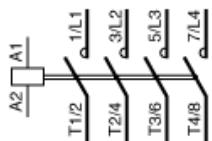
3-Pole Contactors: 3P + N/C
