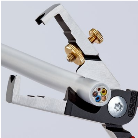
Induction-hardened shear blade with precisely ground cutting edges for crush-free cutting of copper and aluminium Lock nut prevents any unintentional adjustment cables of up to Ø 15 mm (5 x 2.5 mm 2 )
