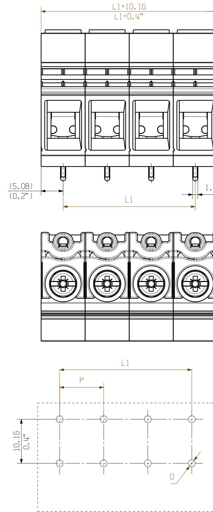
For the mounting of PCBs, it should be noted that the rated data given in the catalogue relates only to the connection elements. The necessary creepage and clearance paths must be observed in connection with the respective applicant in accordance to VDE 0110. The current-carrying capacity and pitch tolerance is to be determined according to DIN IEC 326 part 3 very fine.
