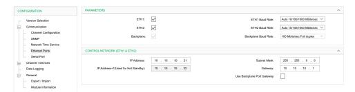
**NOTE:** This option is only available and take effect on the module PV>=04 (with front ethernet port) and using BMENOR2200H.3 from Device list for configuration.
