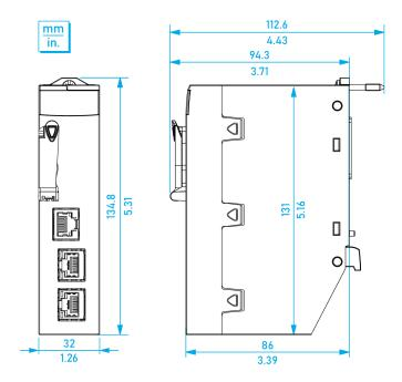
Module mounted on rack:
