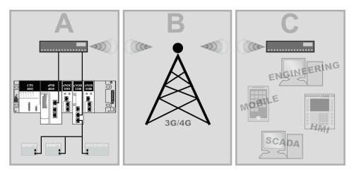
**A** A BMENOR2200H module communicates over the backplane Ethernet port and/or the front control ports with a controller that is connected to a network router.
