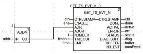
**NOTE:** Read one event in a single PLC cycle for each time stamping module. When the DONE parameter turns to TRUE, the event has been read and stored in the buffer. You can move to the next step.
