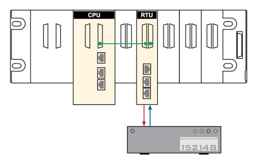
**red line:** The BMENOR2200H module sends an SNTP request over ethernet port to the SNTP server.
