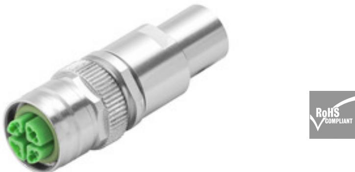
The 8pole M12 Mini crimp cable connector with X-coding and 90° cable exit is with compact dimensions and 8 cable exit positions predestined for difficult installation conditions. The cable clamp version with the wide cable clamp ranges from 4 up to 9 mm plus the fully shielded housing together with the shielded strain relief is the universal fail-safe solution for all common cables on the market.
