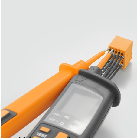
Maintenance through test tap
