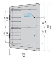
(1) 2 tapped entries for  $n^{\circ}$  16 (Pg 16) cable gland. For ISO M20, use adaptor DE9RA620.
