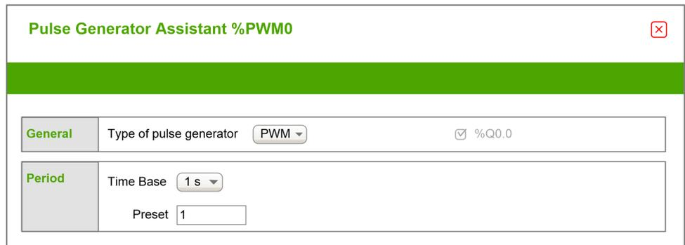
The table describes each parameter available when the channel is configured in **PWM** mode:
